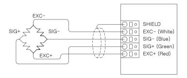
Because wire color may be different according to a manufacture and load cell models. Please refer for the data sheet of load cell. The wire color of load cell according to a manufactures.
