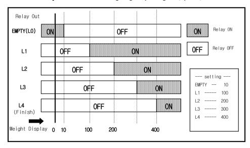
Relay mode 3: Discharge weighing output signal (external)
