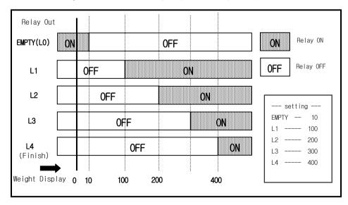
Relay mode 3: Discharge weighing output signal (external)
