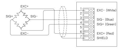
The wire color of load cell according to a manufactures.
