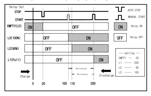
Relay mode 4: Comparator weighing output signal
