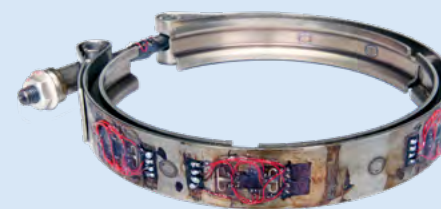
Strain Gauge Application on Clamp
