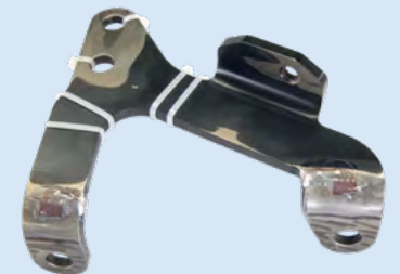
Strain Gauge Application on Holding Bracket
